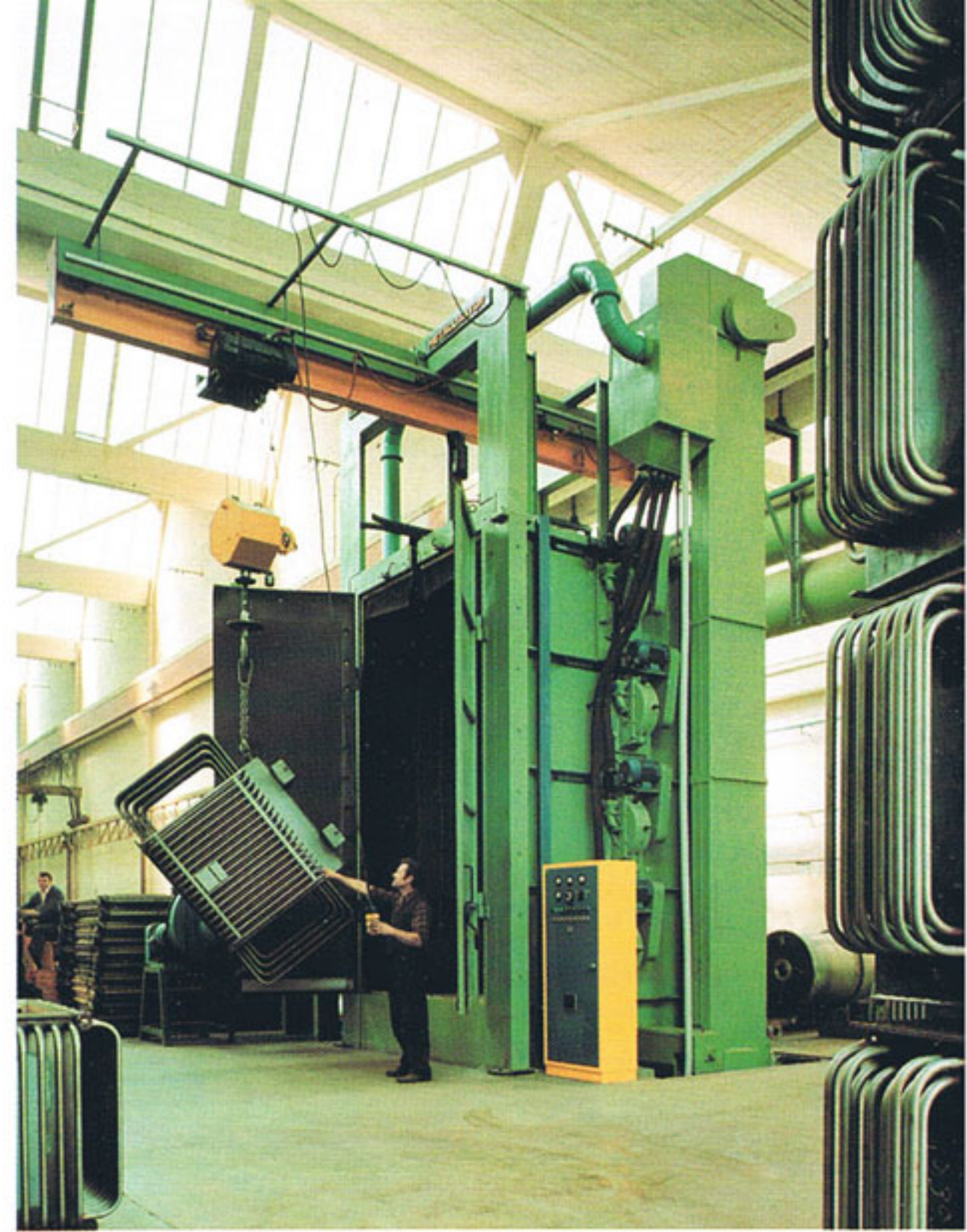
GRANIGLIATRICI A PARANCO. PORTATA 2 ÷ 15 TON HOIST SHOTBLAST UNITS. CAPACITY 2 ÷ 15 TONS GRENAILLEUSES A PALAN. CAPACITE 2 ÷ 15 TONS
