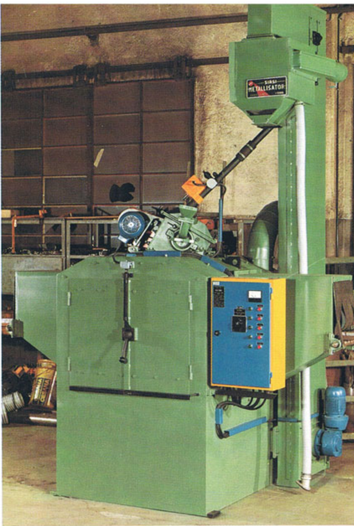
GRANIGLIATRICI A TAVOLA ROTANTE. Ø 1100 ÷ 2300 ROTARY TABLE SHOTBLAST UNITS. Ø 1100 ÷ 2300 GRENAILLEUSES A TABLE ROTATIVE. Ø 1100 ÷ 2300
